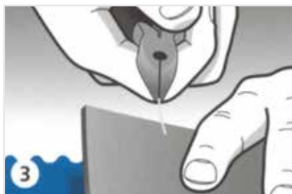
Gently pull the pin out using pliers.
