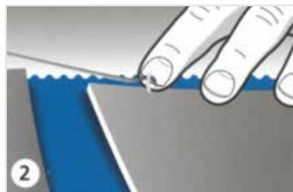
Pop the pin out at 1.5 cm from the edge.
