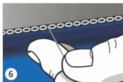
Pass the wire through and cut the excess.
